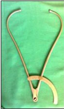
**Fig (1): Manual spreading caliper**
