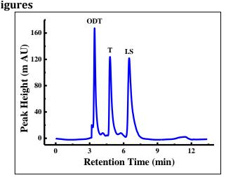
Figure (3): Chromatogram for one calibrator 1000ng/ml
