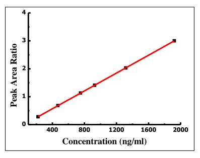
Figure (B): Tramadol calibration curve on HPLC
