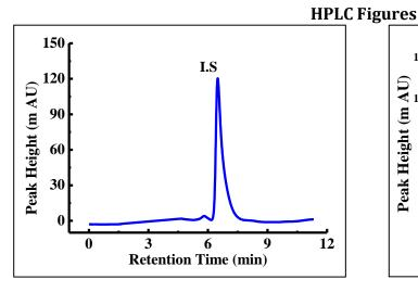
Figure (2): Chromatogram for negative quality control (blank urine)
