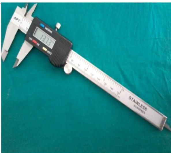
**Fig (1): Electronic digital caliper**
