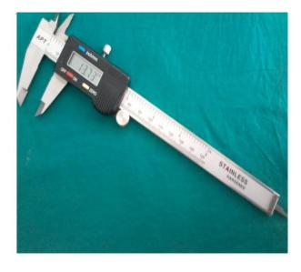
Fig (1): Electronic digital caliper
